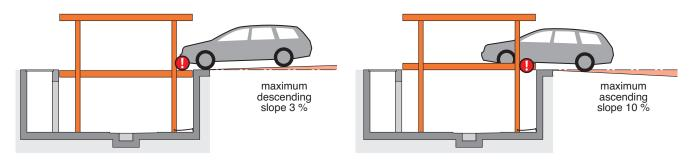
The illustrated maximum approach angles must not be exceeded. Incorrect approach angles will cause serious maneouvring & positioning problems on the parking system for which the local agency of KLAUS Multiparking accepts no responsibility.
