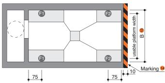
Units are dowelled to the floor. Drilling depth: approx. 15 cm.
