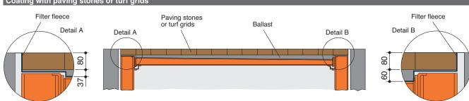
Before paving, the trough must be lined with a water-permeable filter fleece by a specialist company on site. Dimensions rounded.
