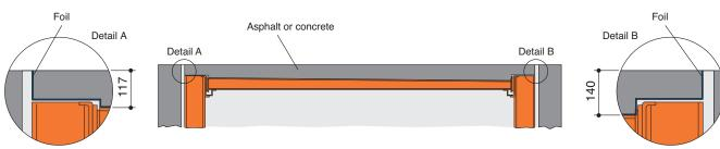
Before filling, the trough must be lined with a water-impermeable foil by a specialist company on site. Dimensions rounded.
