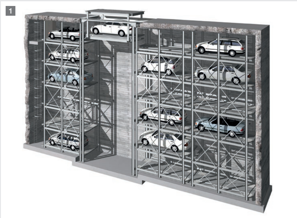
1 MasterVario S with retracting access station
